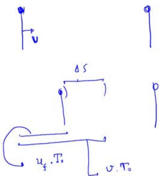
$$T_d = \frac{\Delta S}{v} = \frac{v T_0 - u_f T_0}{v} = \bar{T}_0 \frac{(v - u_f)}{v}$$
